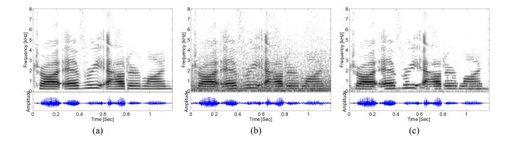
Figure 1: Speech spectograms and waveforms. (a) Clean signal: "Try any other line."; (b) speech corrupted by factory noise with 5 dB SNR (LSD= 6.68 dB, SegSNR= 0.05 dB); (c) speech reconstructed by using 4-state model (LSD= 3.14 dB, SegSNR= 6.76 dB).
